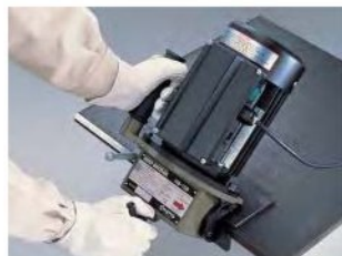
Beveling steel plates
